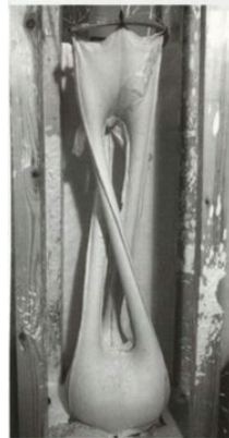
Friedrich Vittzthum Fabric formwork experiment using tension sleeves to restrain the fluid forces of cast concrete
