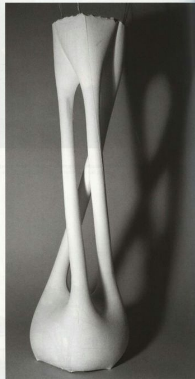
Friedrich Vittzthum Fabric formwork experiment using tension sleeves to restrain the fluid forces of cast concrete
